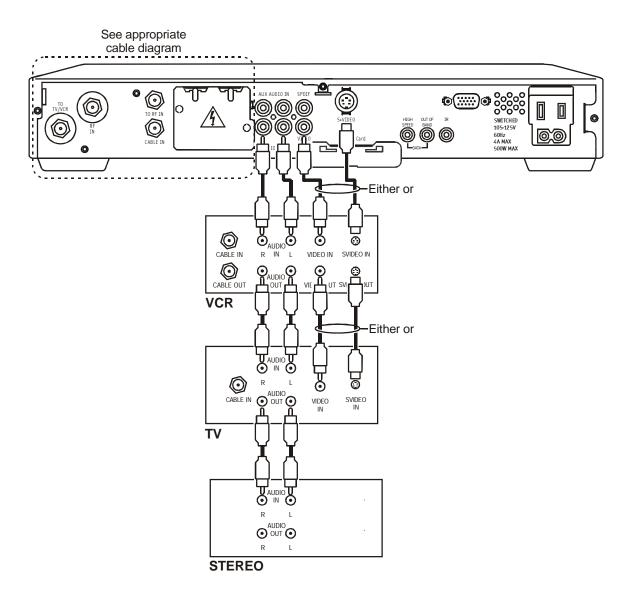
When all of the RCA audio connectors on the back of the stereo receiver are used, the DCT 2000 enables audio to pass through an external device such as a CD player. In this configuration, a subscriber's CD player can be played through the DCT 2000 to a stereo receiver. Figure 3-16 illustrates how to connect the RCA baseband auxiliary audio input/output on the DCT 2000:
