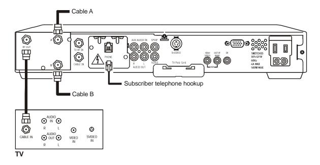
Figure 3-10 illustrates a DCT 2000 with the Dual A/B RF Bypass module when the return is on Cable A:
