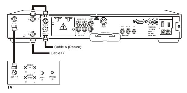
Figure 3-11 illustrates a DCT 2000 with a Dual A/B RF Bypass module when the return is on Cable B:
