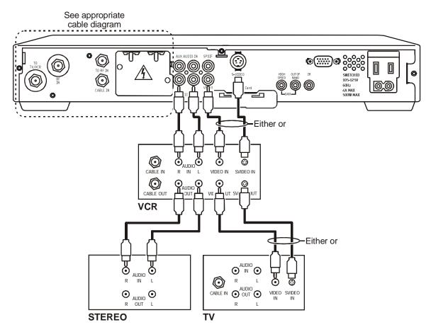
This audio configuration enables the TV to play through the stereo. Figure 3-15 shows how to connect the DCT 2000 to a stereo using the audio loop-through connectors on the VCR and the audio output ports on the TV monitor:
