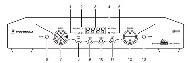
These controls provide minimum, yet functional capability in the event the remote control is lost or temporarily out of service. Functions requiring a numeric entry are not available without a remote control.
