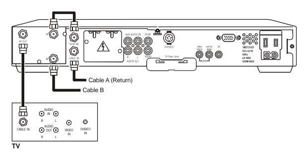
Figure 3-8 illustrates a DCT 2000 when the return is on Cable B:
