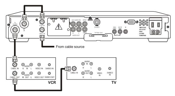
The remodulated channel, 3 or 4 does not carry stereo for digital channels. Connect the DCT 2000 using RCA baseband connectors to receive stereo on digital channels. These connections are illustrated later in this section.
