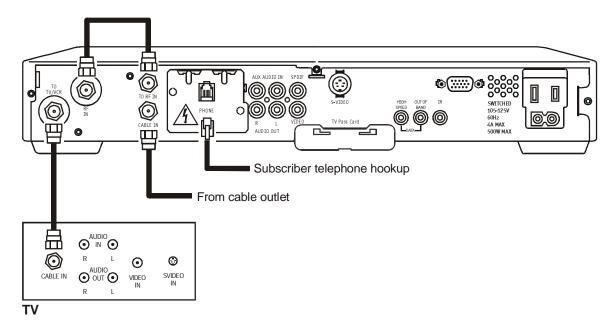
For service providers planning to implement RF return capabilities, it is recommended the DCT 2000 be wired for both the STARFONE telephone return and the integrated STARVUE RF return. This enables the operator to move the DCT 2000 into a two-way RF return without rewiring the DCT 2000 later.
