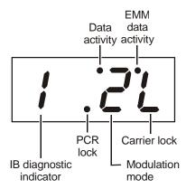
Figure B-7 illustrates the IN-BAND DIAGNOSTIC (in-band receiver digital status) OSD:
