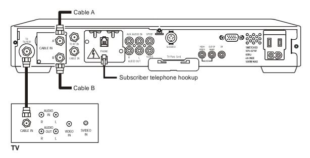
Figure 3-7 illustrates a DCT 2000 with the return on Cable A:
