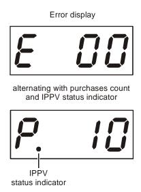
The purchases count is used by Customer Service Representatives (CSRs) to check returned DCT 2000 for uncollected purchases, that are used to close out a subscriber's account. The largest error code takes priority.
