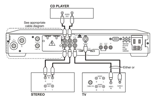
The DCT 2000 must be turned off from the front panel to enable audio loop-through signals to pass through. When the DCT 2000 is powered on, the audio outputs correspond with the currently tuned channel on the DCT 2000.
